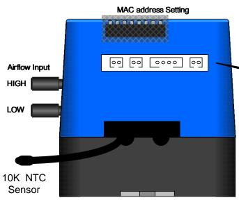
\*Caution: when use 24VAC power, please make sure the power polarity is same with all device, or it may be caused damage.(Half-wave rectification)
